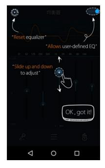
Master EQ switch: Slide the lever on the upper right to the right to activate the equalizer.
